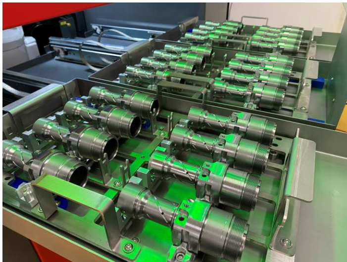
Caption: Product carriers with hydraulic blocks that Intercable Tools will be able to deburr automatically in future using ultrasonic deburring technology from ultraTEC innovation.
