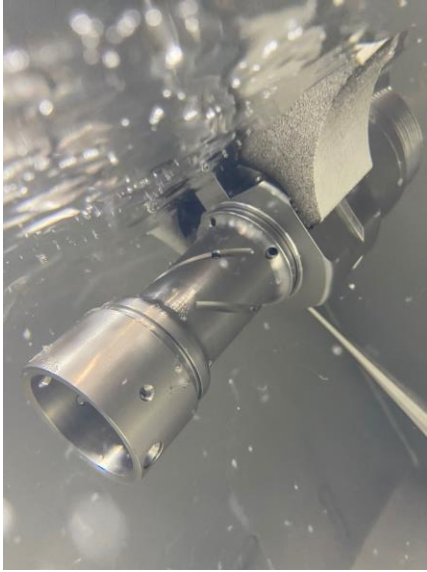
Caption: The process of ultrasonic deburring of the hydraulic blocks uses ultraTEC technology with an ultrasonic sonotrode, whose generated vibrations remove burrs and chamfers in an energy-efficient manner.
